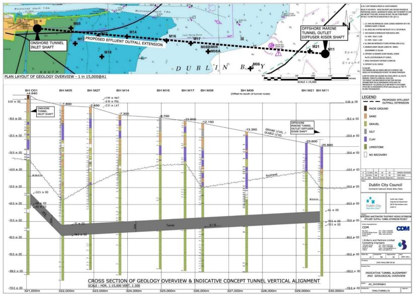
Figure 5: Plan and Cross Section of Tunnel Route
